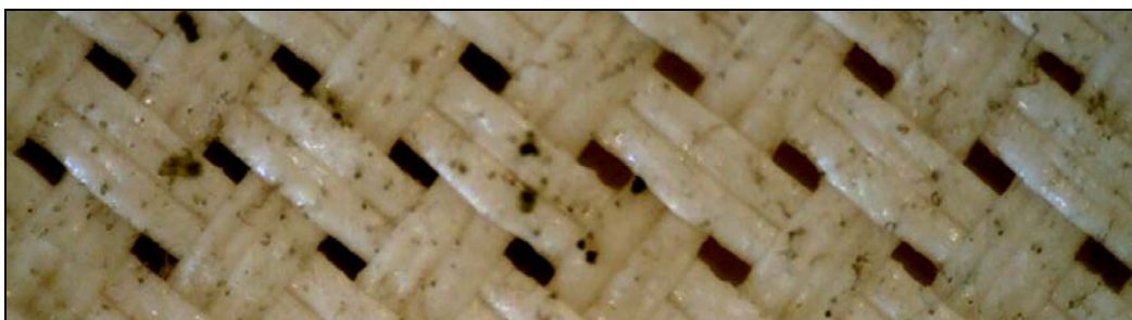
View of sample using the stereoscope – trace growth is visible.
